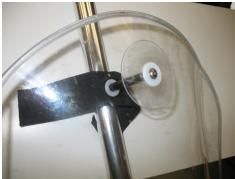
Fig 1. windscreen with reinforcing washer applied to the inner surface.
